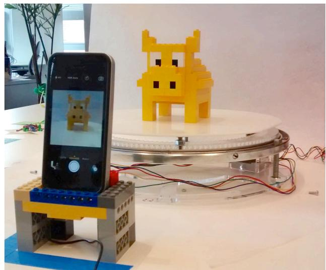
Figure 1: Spin Turntable and Mobile Application
